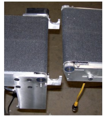
A. Conveyor Sections drop
